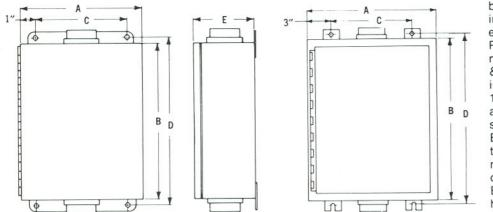
Weatherproof Sheet Steel Multi-circuit box protects thermocouple and instrument cables from corrosive or dirty environments
